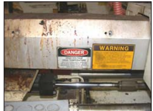
Figure 7. A guard equipped with safety signs covers the barrel of the injection unit.
