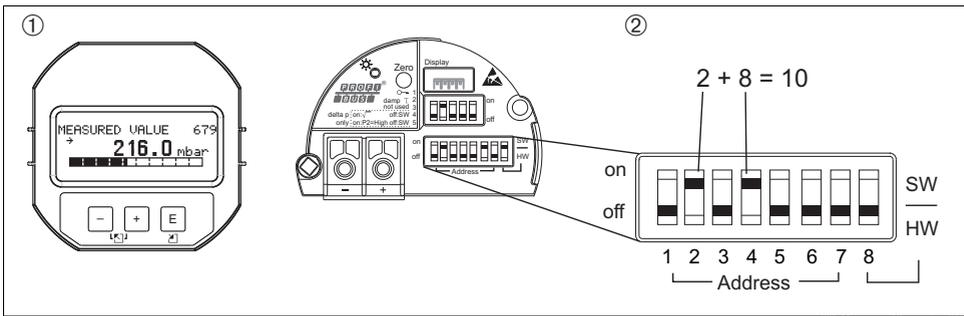
Fig. 6: Setting the device address via DIP switches
