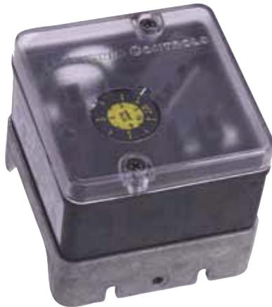
The Model G is a gas pressure switch that monitors pressure and breaks the electrical control circuit when pressure drops below or rises above the desired setpoint. The gas pressure settings are adjustable.
