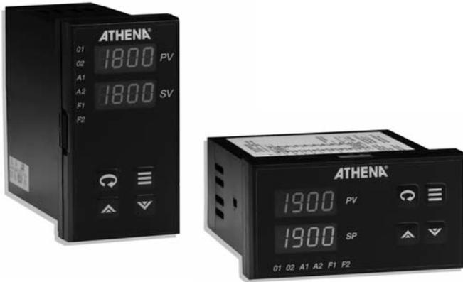
The Athena 18C and 19C are available as 1/8 DIN (18C) vertical or 1/8 DIN (19C) horizontal models. Both panel mounted, auto-tuning controllers can be used for precise control of a single loop with two independent outputs field-configurable as direct acting, reverse acting, and 2 alarms. RS-232 or RS-485 communications interfaces are available for both models, and two digital LED displays provide visual indication of various controller functions.
