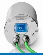
All BON sensors have a display to show to directly monitor the relevant process parameter in real-time. This eliminates the need for operators to be skilled in spectroscopy and able to quickly see when measurements are in spec or not.
