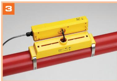
3 Connect power and sensors to electronic assembly
