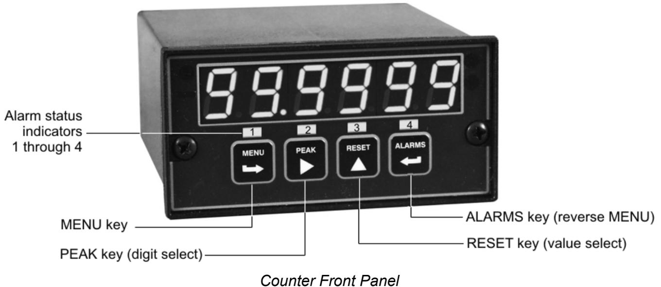
There are four front panel keys, which change function for the **Run Mode** and **Menu Mode**, effectively becoming eight keys. The keys are labeled with alphanumeric captions (MENU, PEAK, RESET, ALARMS) for the Run Mode and with symbols (➡ right arrow, ▶ right triangle, ▲ up triangle, ← left arrow) for the Menu Mode.
