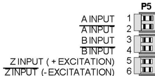
Z input or excitation is jumper selectable. With differential quadrature inputs and an external power supply, connect ground of the external supply to Pin 6 of P1.
