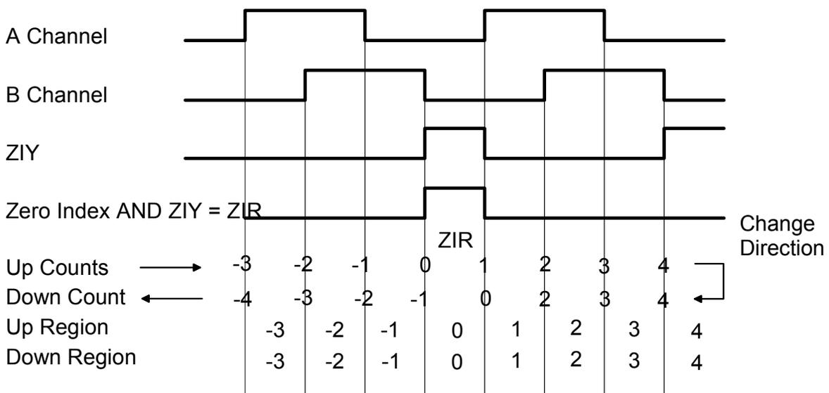
By ANDing the zero index signal with the A & B channels, there is no regional discrepancy between counting up and counting down.
