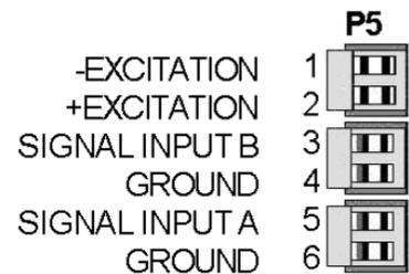
Ground pins 4 & 6 are internally connected.
