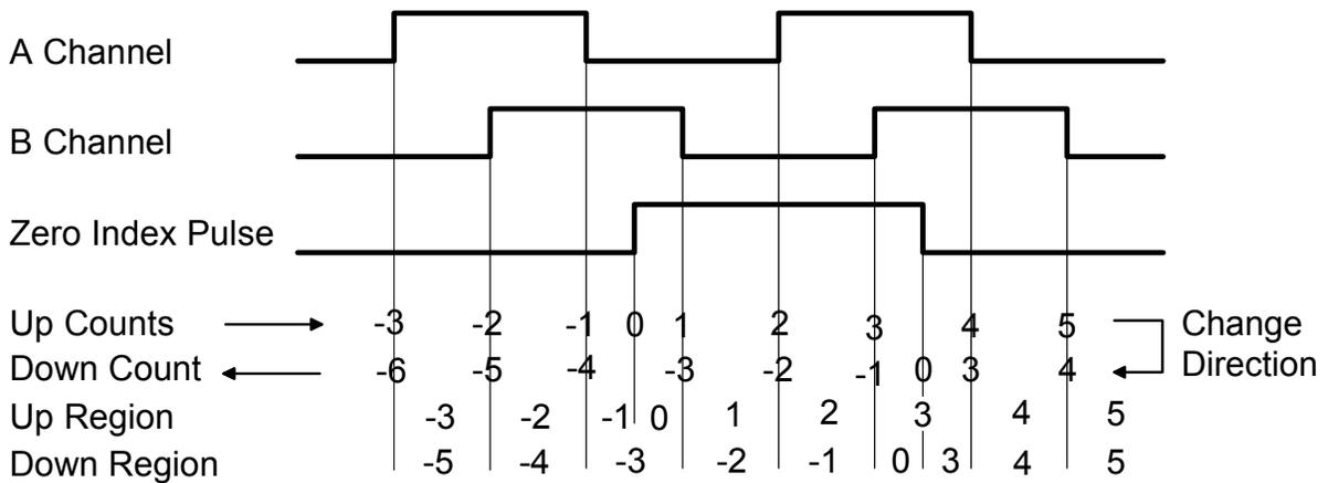
It follows that a wide zero index signal causes a discrepancy in the count in the regions between transitions when counting up and counting down. To correct this situation, AND the zero index signal with the A & B channel signals. Assume for this example the zero index is ANDed with the inverse of A ( $\bar{A}$ ) and the inverse of B ( $\bar{B}$ ) to produce ZIY as shown below.
