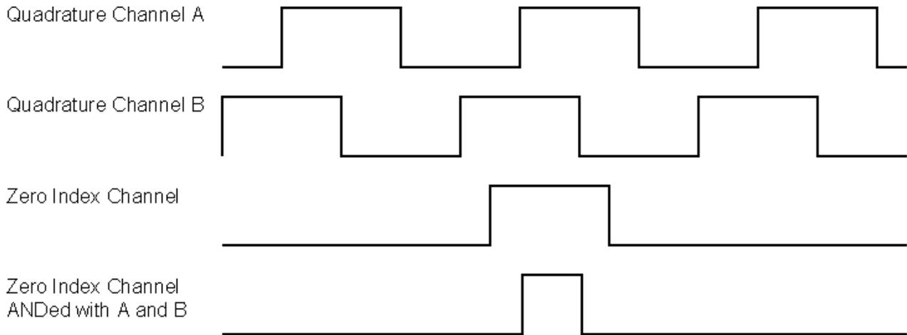
Our quadrature signal conditioner board can be used for quadrature position (with Basic or Extended main board) or for quadrature rate (with Extended main board). Two quadrature signals, which are 90° out of phase, are applied to the Channel A and B inputs. Their phase relationship determines whether the count is up (+) or down (-). A zero index signal may be applied to Channel Z as a position reference.
