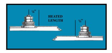
Post terminals are located 1/4" from edge of heated section.
