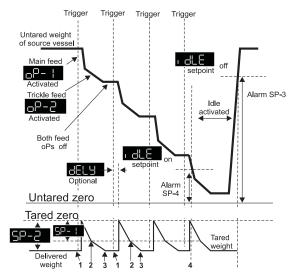
Typical Loss of Weight Application with Idle Function
