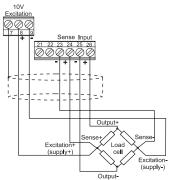
Single Load Cell Transducer Connections with Remote Sense
