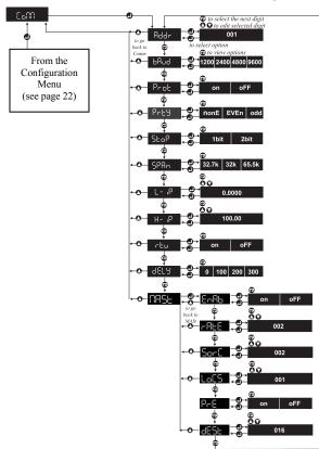
The instrument can use 3 prototcols:
