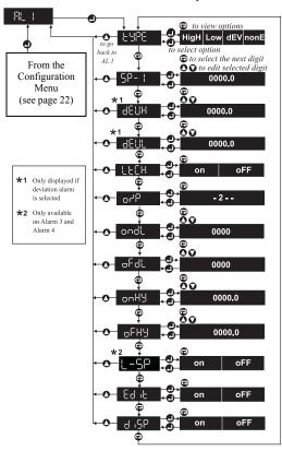
Each alarm can be high or low acting or a deviation alarm. When an alarm occurs:
