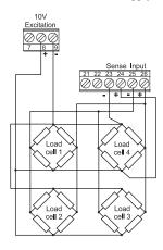
Multiple Load Cell Transducer Connections
