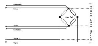
The load cell wiring above shows a 6-wire connection. If sense wires are not available from the load cell (4-wire system), link Terminals 9 to 23 and Terminals 8 to 24.
