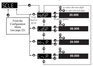
If the system is calibrated to known weights as described above, do not change **H-ip** and **L-ip**. Enter weights for **HdSP** and **LdSP** only.
