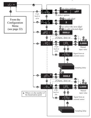
Between 2 to 8 calibration points may be defined in terms of load cell input (mV/V) and the corresponding displayed value. A 3-point relationship is illustrated below.
