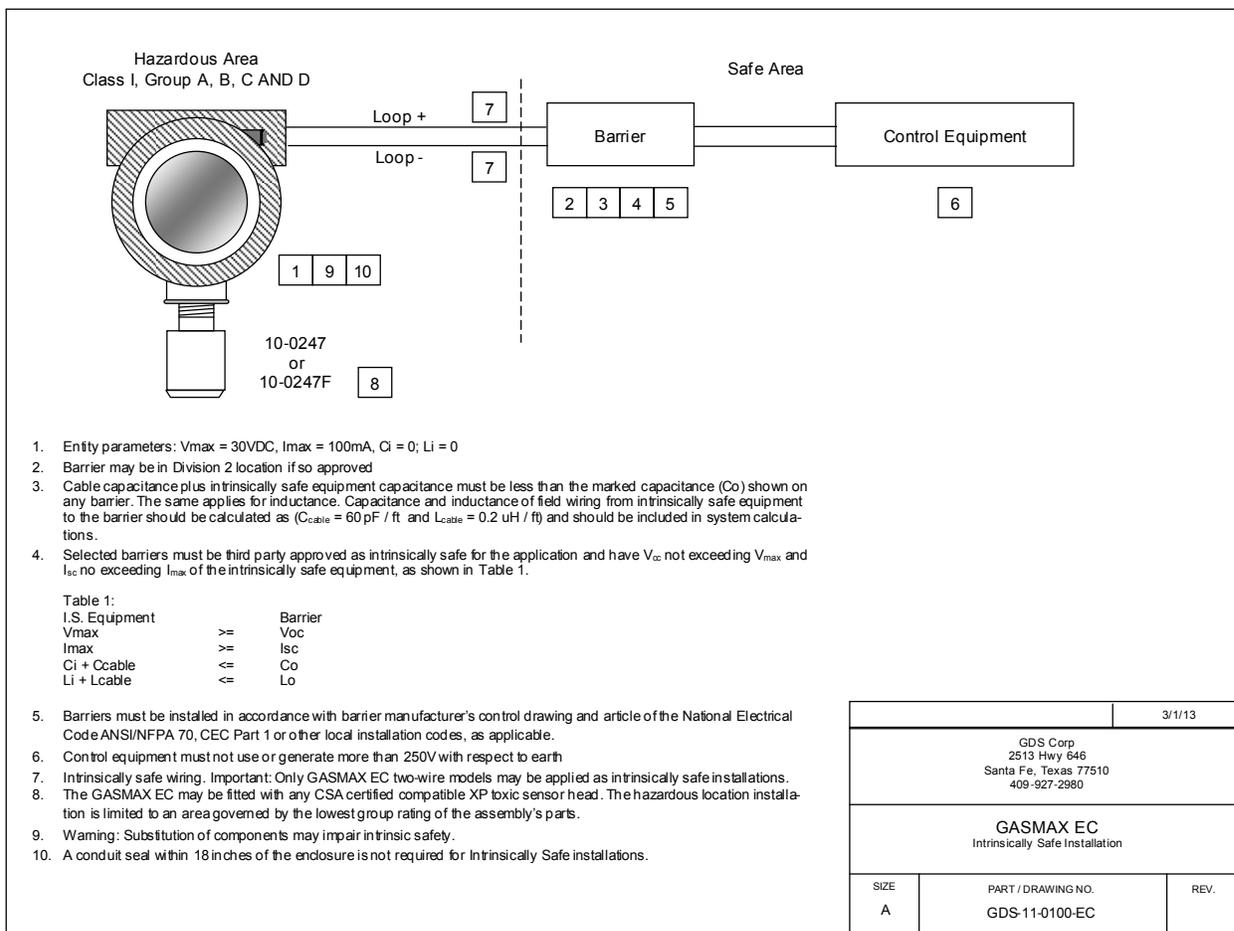
Figure 4-6: GASMAX Intrinsically Safe Installation
