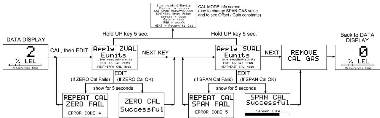
Figure 5-2: CALIBRATION FLOWCHART
