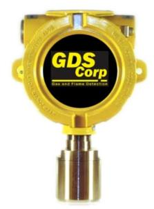
The GDS-50 is a three-wire remote sensor transmitter designed specifically to detect combustible hydrocarbons or carbon dioxide gas. The GDS-50 sensor transmitter 4-20mA output is compatible with the C1 *Protector*, C2 *Protector*, C2 *Quad Protector* or C64 *Protector* Controllers, the GASMAX II or GASMAX CX gas monitors or any other device with a 4-20mA input and built-in calibration capability.
