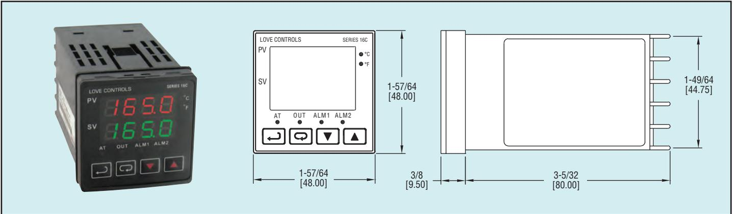
The compact Series 16C Temperature Controller offers accurate temperature measurement and control in a 1/16 DIN package. Designed for direct or reverse acting (cooling or heating) control, the Series 16C can be programmed for simple ON/OFF or more complex PID control functions. PID control is supported with manual or auto-tuning. Select relay, voltage or current output for control methods.
