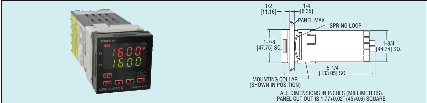
The **16L Series Temperature/Process FM Approved Limit Controls** set a new standard in 1/16 DIN limit controls. The 16L offers universal input (10 thermocouple types, 4 RTD types, voltage, and current), single set point or dual set point. Standard features include remote reset capability, peak/valley indication, open sensor protection, input rate of change protection, and much more.
