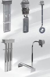
Fluoropolymer (PTFE) Heaters: Compatible with virtually any chemistry. Sizes up to 18 kilowatt. Single or three phase. Large variety of standard and custom configurations for over-the-side and tank bottom installations. Low profile, custom designs available. Rigid and flexible risers available. Screw plug and flange heaters in sizes from ½-inch screw plug (100 watt) to 6-inch flange (18 kW). Thermal overtemperature protection standard (except screw plug). cULus and CE.
