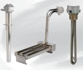
Metal Heaters: Variety of materials to match your application (titanium, 316 and 304 stainless steel, and plain steel). Sizes up to 54 kW. Standard and custom configurations for over-the-side and bottom installations in open tanks. Screw plug and flange heaters in titanium and 316 stainless, sizes from ½-inch screw plug (100 watt) to 6-inch flange (72 kW). Thermal overtemperature protection standard (except screw plug). cULus and CE.
