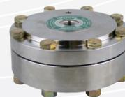
High Displacement seals are used with pressure instruments that require a high fluid displacement in order to actuate the instrument (e.g. Mechanical DP Gauges). The extra large diaphragm also makes these seals useful for low pressure gauges and high accuracy transmitter assemblies.
