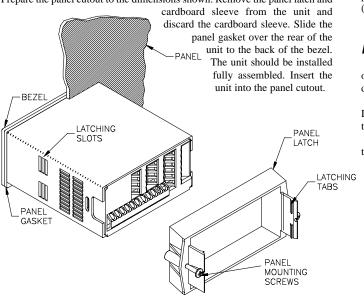
While holding the unit in place, push the panel latch over the rear of the unit so that the tabs of the panel latch engage in the slots on the case. The panel latch should be engaged in the farthest forward slot possible. To achieve a proper seal, tighten the latch screws evenly until the unit is snug in the panel (Torque to approximately 7 in-lbs [79N-cm]). Do not over-tighten the screws.
