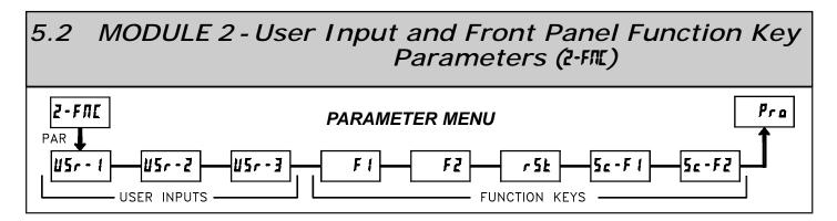
The three user inputs are individually programmable to perform specific meter control functions. While in the Display Mode or Program Mode, the function is executed the instant the user input transitions to the active state.
