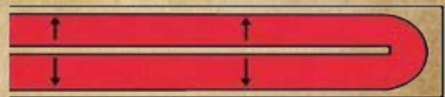
Watt-Flex ® heater halves expand independently
