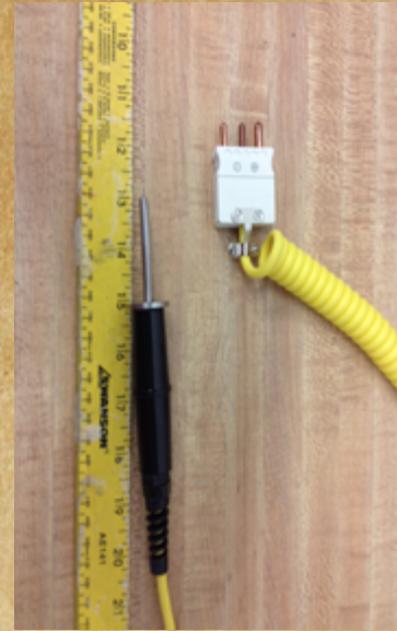
SP-1850 RTD for measuring temps on dog treats
