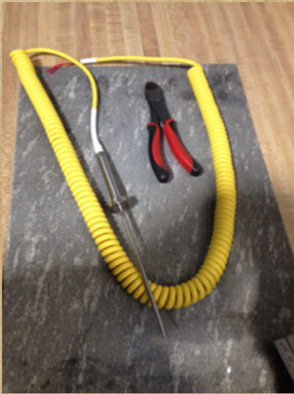
SP-1853 2252 Ohm Thermistor with S.S. handle
