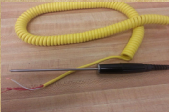
SP-1669 & SP-1427 & SP-1324 RTD Banana Probe & Cookie Dough Probe
