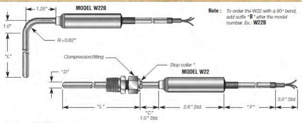
\* No stop collar option , " C " = N00 Stop collar recommended for temperature above 100°C
