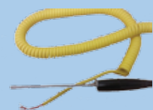
RTD PENETRATION PROBE (nylon handle)
