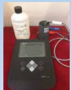
W.H. COOKE #PPG-CT55-KIT-REV3 E-COAT CONDUCTIVITY KIT: Includes benchtop pH meter, conductivity cup, automatic temperature compensation probe, 3 ft. quick disconnect jack & banana plugs, 500ml conductivity standard.
