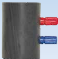
CT-55 CONDUCTIVITY CUP FOR E-COAT PAINT PROCESS
